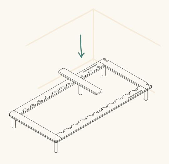
Secure together using 2x frame hand screws with washers.
