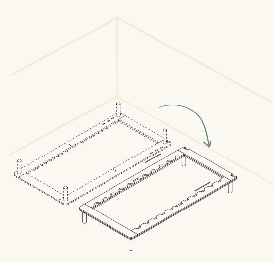
Place previously assembled section onto frame.
