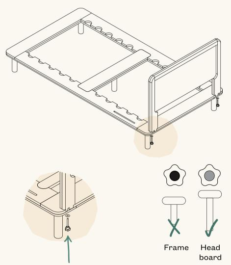
Secure back of headboard using 2x headboard hand screws.
