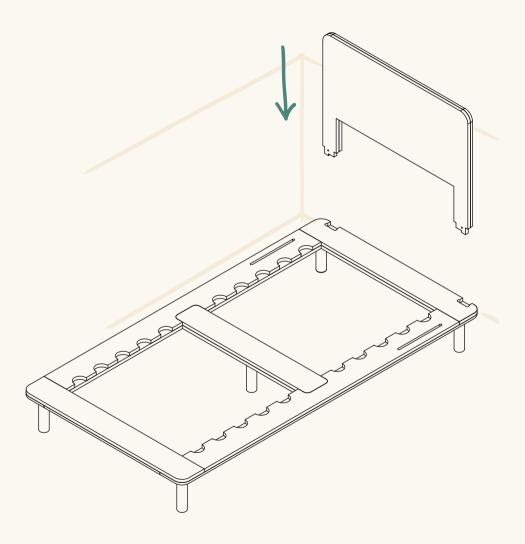
Secure bottom of headboard using 2x washers and headboard hand screws.
